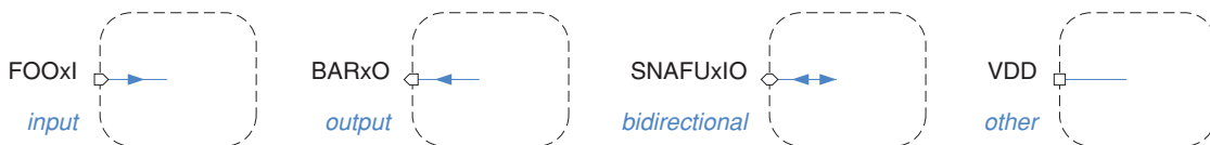
Fig. 5.11 Terminals in schematic diagrams.
