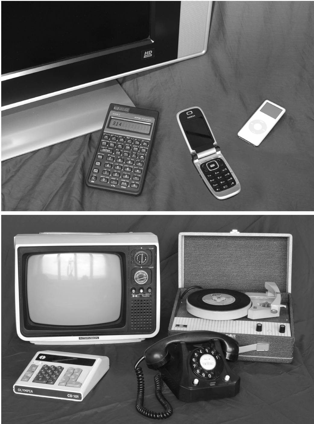
Fig. 1.2 Four electronic products that take advantage of microelectronics opposed to analogous products that do not. The antiquated devices operate with vacuum tubes, discrete solid-state devices, and other electronic components but include no large-scale integrated circuits. Also observe that, were it not for display size and audio volume, one might replace all four devices with Apple's iPhone that has brought seamless system integration to even higher levels (photos courtesy of Alain Kaeslin).
